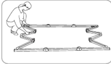
11. Again, press in the silver locking buttons. Then, pick up one end of the folding frame, and walk it to the other end, folding the longer sections into thirds.
