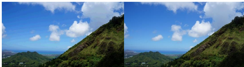
In these simulated images, insufficient grayscale rendition (left) causes horizontal banding in the sky. This artifact is absent in the image on the right.
