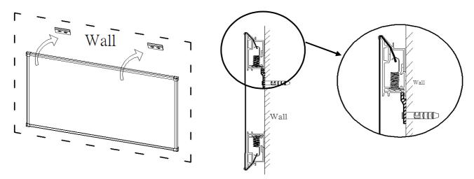
**Step 16:** With the frame slightly tilted outward; connect the bottom brackets onto the bottom groove of the frame. Then secure them by screwing onto the wall
